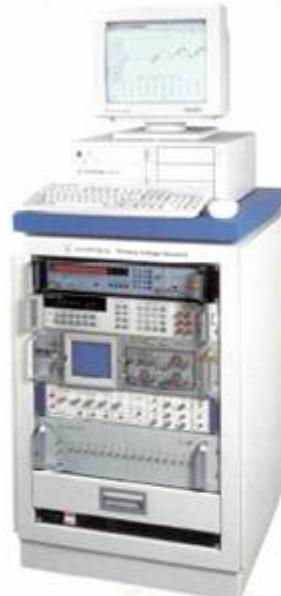
The **HYPRES** Primary Voltage Standard System is a complete, computer controlled system to implement a variety of voltage calibration functions. Using this system, secondary voltage standards and voltmeters can be calibrated automatically. A properly used Josephson Standard is correct by definition because of its realization of a quantum physics phenomenon, and the adoption of that phenomenon as the basis of the SI Volt representation.
