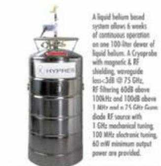
A liquid helium based system allows 6 weeks of continuous operation on one 100-liter dewar of liquid helium. A Cryopump with magnetic & RF shielding, waveguide lens-3dB @ 75 GHz, RF filtering 60dB above 100Hz and 100dB above 1 MHz and a 75 GHz diode RF source with 1 GHz mechanical tuning, 100 MHz electronic tuning, 60 mW minimum output power are provided.
