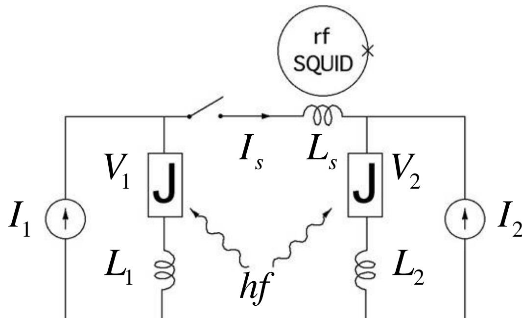
$$I_s = \frac{1}{L} \int (V_1 - V_2) dt$$
