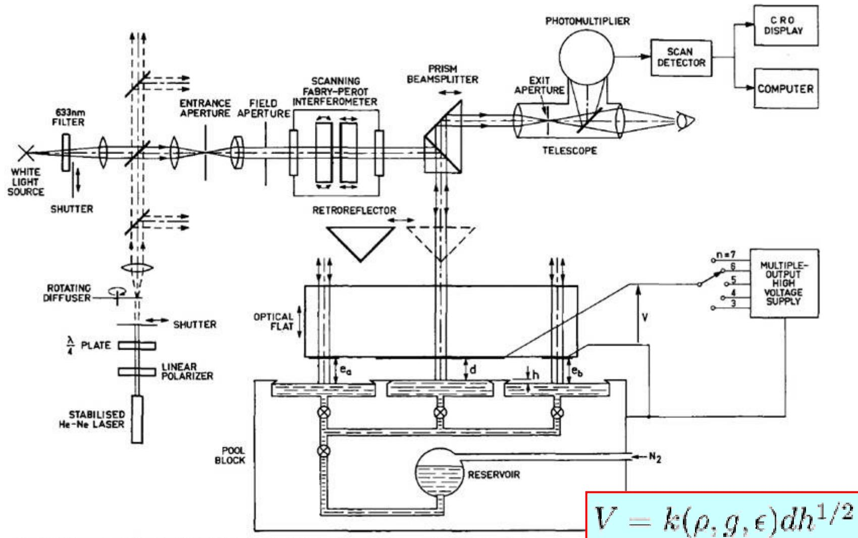
Fig. 1. Schematic of absolute liquid electrometer and optical measuring system
