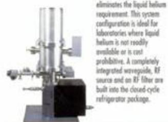
A closed-cycle refrigerator based system allows continuous operation and eliminates the liquid helium requirement. This system configuration is ideal for laboratories where liquid helium is not readily available or is cost prohibitive. A completely integrated waveguide, RF source and an RF filter are built into the closed-cycle refrigerator package.
