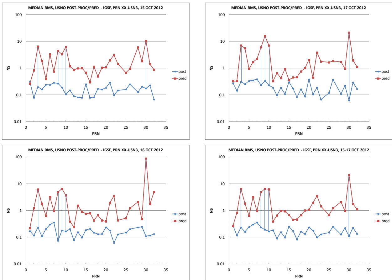
Figure 6. RMS error of USNO clock estimates, post-processed (“post”) and predicted (“pred”), each day of 15-17 Oct 2012 and overall. Vertical lines mark PRNs 3, 8, 9, 10 and 30. Prediction error does not seem correlated with error of post-processed values.
