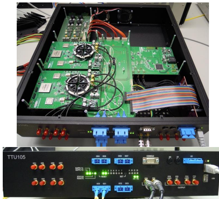
Figure 1. The recently developed 2U (90 mm) time transfer unit hardware. Front panel and top view (without cover). See [7] for details.
