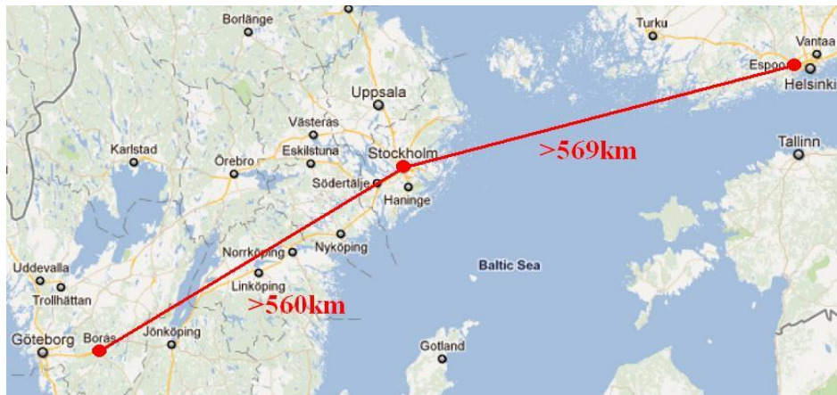
Figure 1. The red lines symbolize the fiber distance from SP (Borås, Sweden) through STUPI (Stockholm, Sweden) to MIKES (Espoo, Finland) with a total length longer than 1129 km. Approximately half of the fiber length is located on the seabed of the Baltic Sea.
