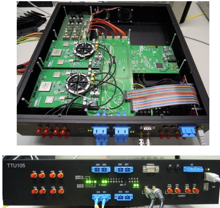
Figure 2. The recently developed 2U (90 mm) time transfer unit hardware. Front panel and top view (without cover). See [7] for details.
