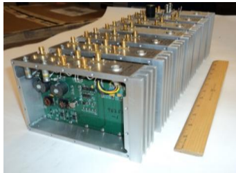
Figure 10. Ion clock assemblies engineered for low power and validation prior to integrated design.
