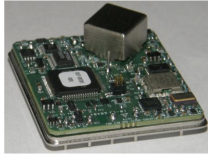
(a) (b) Figure 3. SA.45s (a) sealed and (b) with lid removed.
