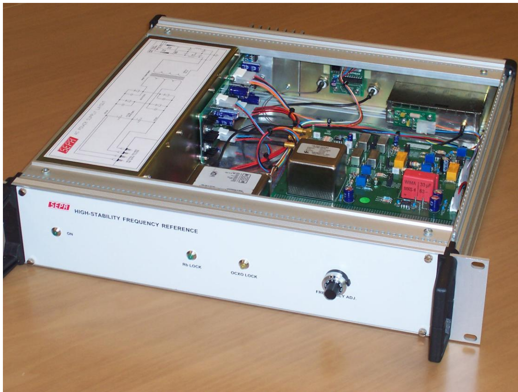
Figure 7. High-stability frequency reference, inner view showing Rb and OCXO.
