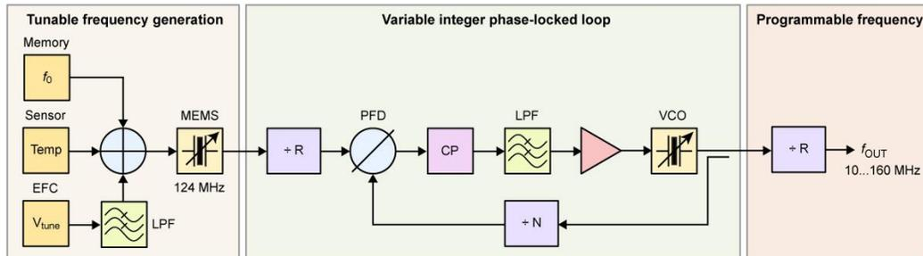
Fig. 1. Block diagram of the temperature-compensated MEMS oscillator (TCMO™) consisting of three functional blocks: tunable frequency generation, variable integer phase-locked loop, and programmable frequency output.
