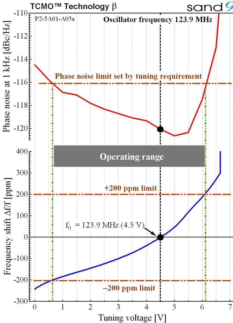
Fig. 6. Result of the frequency tuning of the MEMS oscillator and dependence of the 1 kHz phase noise versus the tuning voltage from 0 to 7 V measured with an Agilent E5052B signal source analyzer.
