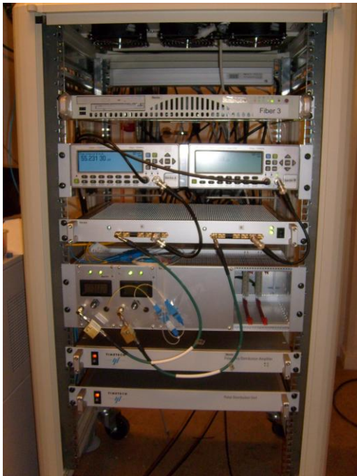
Figure 10. The present system requires several individual pieces of equipment connected by external cables at each node: (to the left) a personal computer with measurement hardware and software at the top; further below two time-interval counters, dual-channel header recognition (HR) box, optical-to-electrical converters, and distribution units for frequency and time pulses at the bottom; (to the right) the custom-made HR-card generates an electrical pulse each time it detects the known sequence of A1 and A2 bytes, and contains a Field Programmable Gate Array (FPGA).
