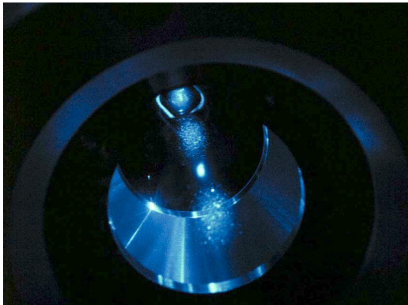
Figure 3. Emission of Sr atoms trapped by a laser cooling technique.
