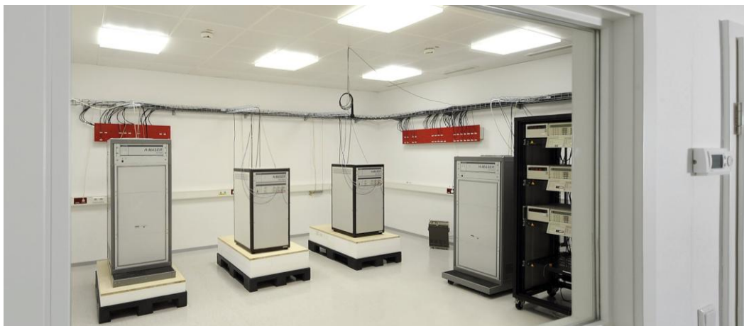
Figure 5. PTB's new clock room hosting four masers and 5071A cesium clocks.
