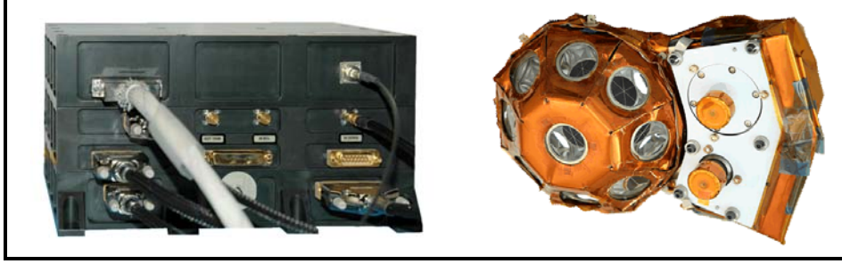
Figure 2. T2L2 flight model: the electronic unit (left) and optical units together with the LRA (right).
