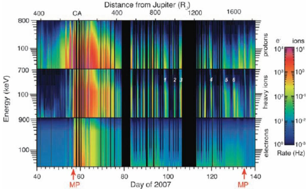
Figure 12. Spectrogram data from the NH s/c Pluto Energetic Particles Spectrometer Science Investigation, PEPSSI Instrument; **MP** indicates spacecraft crossing of Jovian magnetopause.<sup>2</sup>
