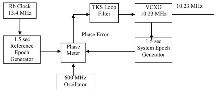
Figure 1. Simplified TKS block diagram.
