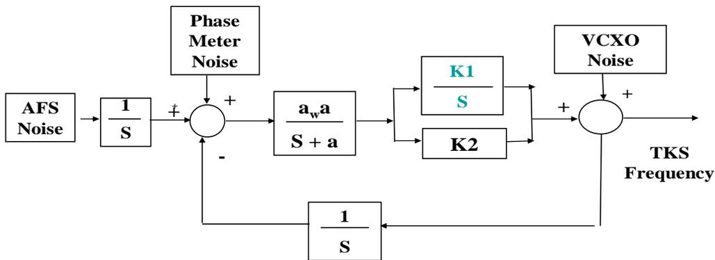
Figure 3 Simplified TKS Error Model in S Domain
