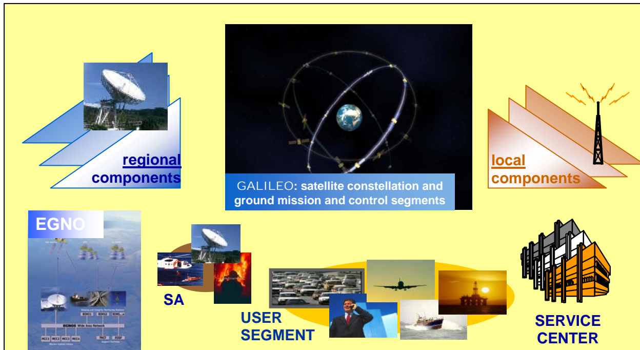
Figure 1. Overall Galileo System overview.
