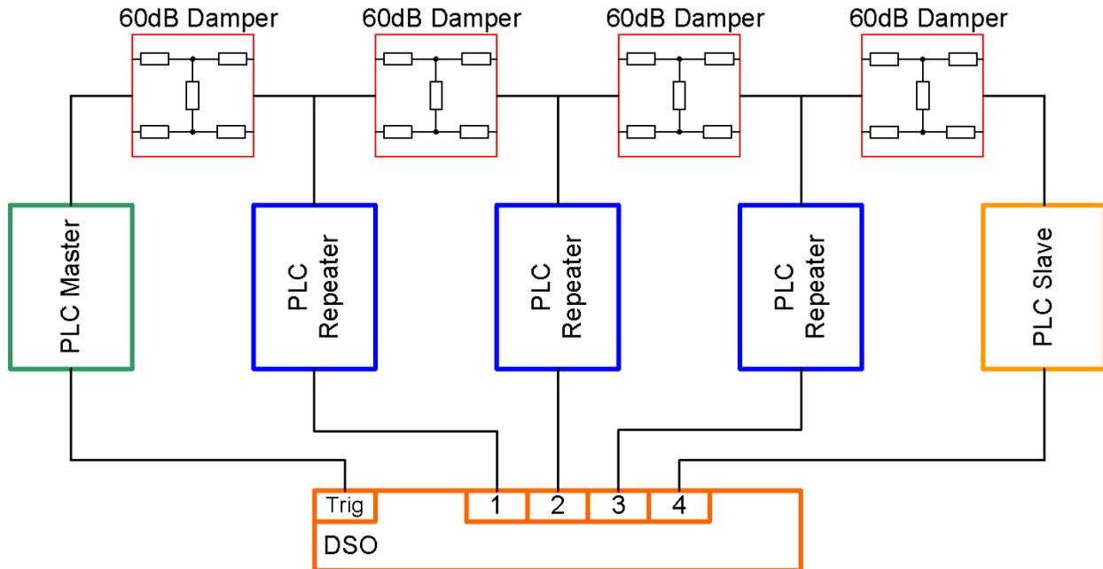
Figure 6. Test setup for PLC.
