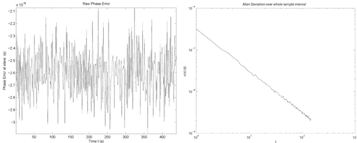
Figure 4. Phase error in the stable case and Allan deviation for the stationary case.
