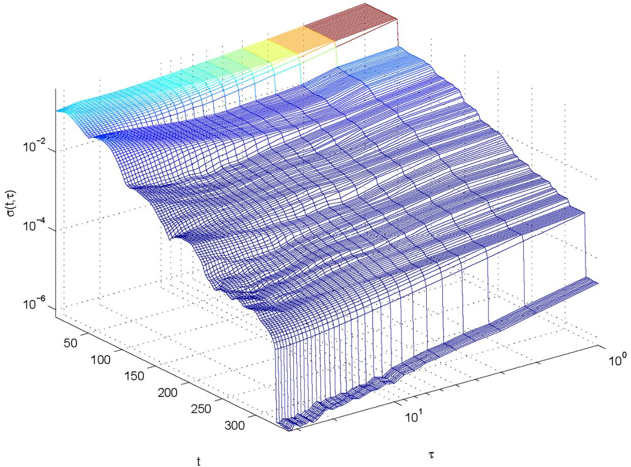
Figure5. Dynamic Allan deviation during power-up.
