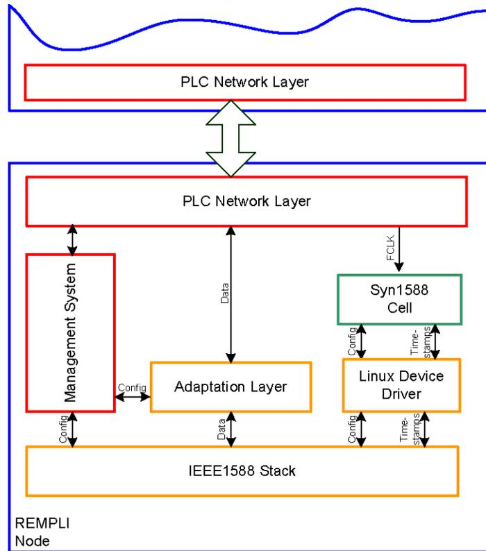
Figure 2. Integration of the adaptation layer into the REMPLI node structure.
