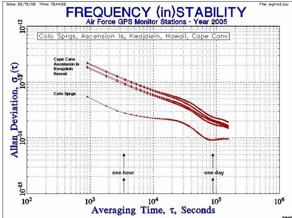
Figure 2. Frequency stability plots of the “clocks” at five of the six AF monitor stations. The AF station at Colorado Springs (Schriever AFB) is tied to the USNO/AMC. The remainder of the AF stations each has two cesium frequency standards.
