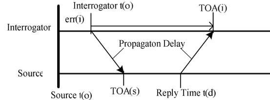
Fig. 1 Message exchange of RTT process
