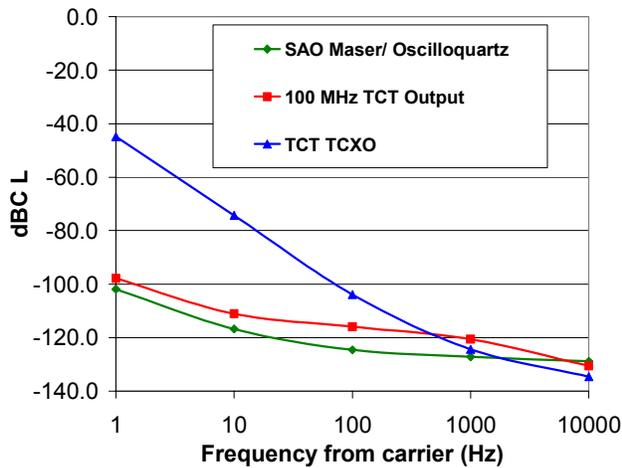
Figure 4. System phase noise at 100 MHz
