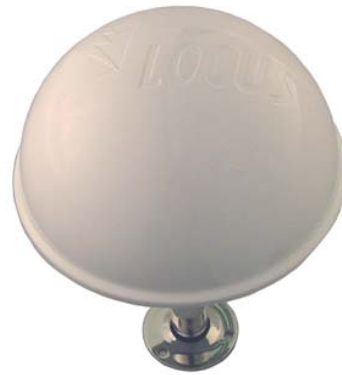
Figure 3. eLoran magnetic or H-field antenna. H-field antennas offer the potential of indoor Loran reception, and these small (< 20 cm diameter and 10 cm height) devices do not require a ground, which also simplifies installation.
