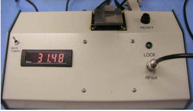
Figure 7. Prototype MAC Installed in test fixture
