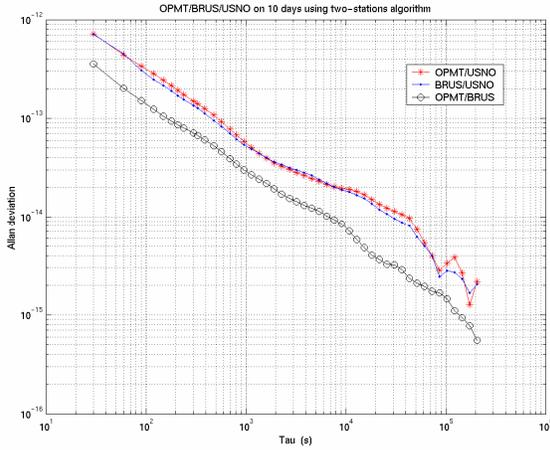
Figure 7. Frequency stability (Allan deviation) of the clock solution obtained with the two-station algorithm on OPMT/USNO, BRUS/USNO and OPMT/BRUS baselines
