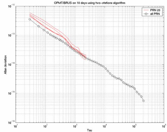
Figure 5. Comparison of the stability of the different passes with PRN 20 to overall clock solution stability on OPMT/BRUS baseline
