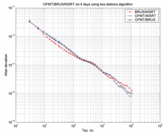
Figure 3. Frequency stability (Allan deviation) of the clock solution obtained with the two-station algorithm on BRUS/WSRT, OPMT/WSRT and OPMT/BRUS baselines
