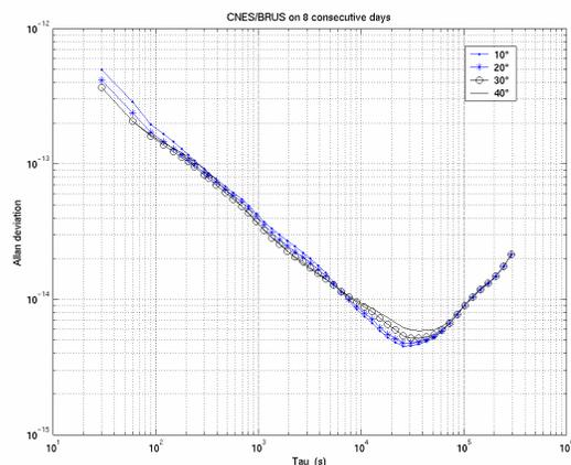
Figure 1. Frequency stability (Allan deviation) of the clock solution obtained with the two-station algorithm on BRUS/CNES baseline for different elevation limitations
