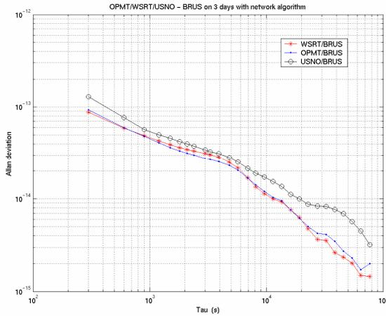
Figure 10. Frequency stability (Allan deviation) of the clock solutions obtained with the network algorithms (Network : OPMT/USNO/BRUS/WSRT)
