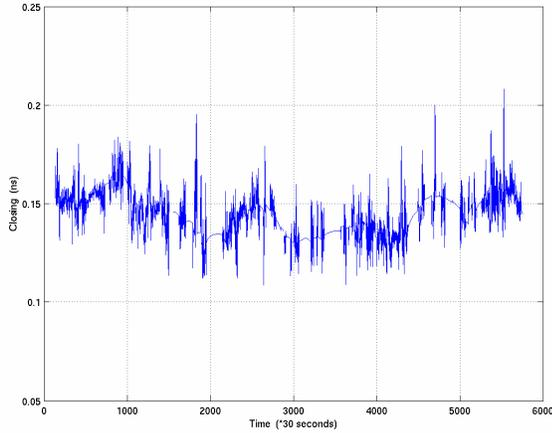
Figure 4. Closing of the clock solutions obtained with the two-station algorithm on OPMT/WSRT, OPMT/BRUS BRUS/WSRT baselines
