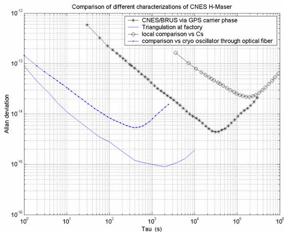
Figure 2. Different characterizations of CNES Hydrogen Maser
