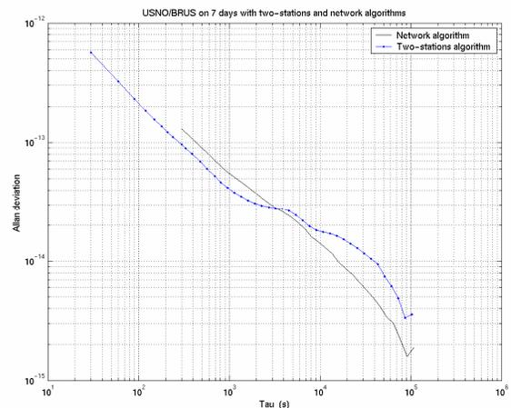
Figure 9. Frequency stability (Allan deviation) of the clock solutions obtained with both algorithms on USNO/BRUS baseline on 7 days (Network : OPMT/USNO/BRUS/ALGO)
