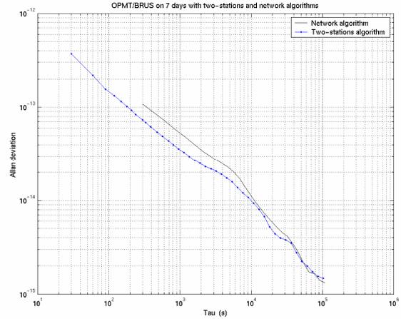
Figure 8. Frequency stability (Allan deviation) of the clock solutions obtained with both algorithms on OPMT/BRUS baseline on 7 days (Network : OPMT/USNO/BRUS/ALGO)
