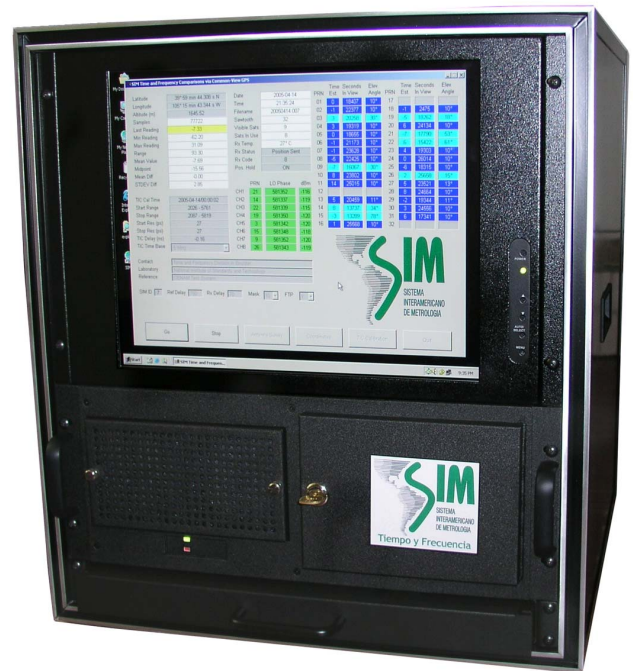
Figure 2. The SIM common-view GPS measurement system.
