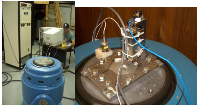
Figure 3. On the left is the vibration table (shaker), amplifier for driving shaker (the vertical rack-mount system), and controller, signal generator, and data-acquisition system in front of operator. On the right is the 10 MHz OCXO device under test (DUT) mounted to the shaker platform.
