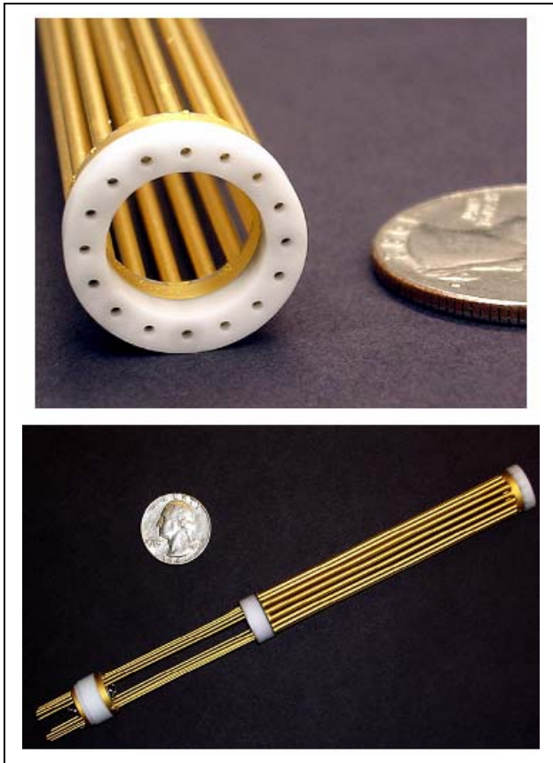
Figure 1. The quadrupole trap for ion optical pumping state selection is on the left and the 16-pole trap where the 40.5 GHz clock interrogation is made is on the right.
