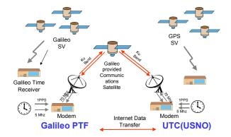
Figure 1. Proposed Setup for GGTO Implementation Phase 1
