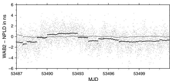
(c) Epoch-wise solution using only code data (gray dots), continuous solution using only phase data (gray line), and daily independent solution using code and phase data (black line).
