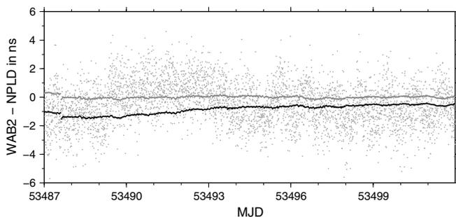
(d) Epoch-wise solution using only code data (gray dots), continuous solution using only phase data (gray line), and continuous solution using code and phase data (black line).
