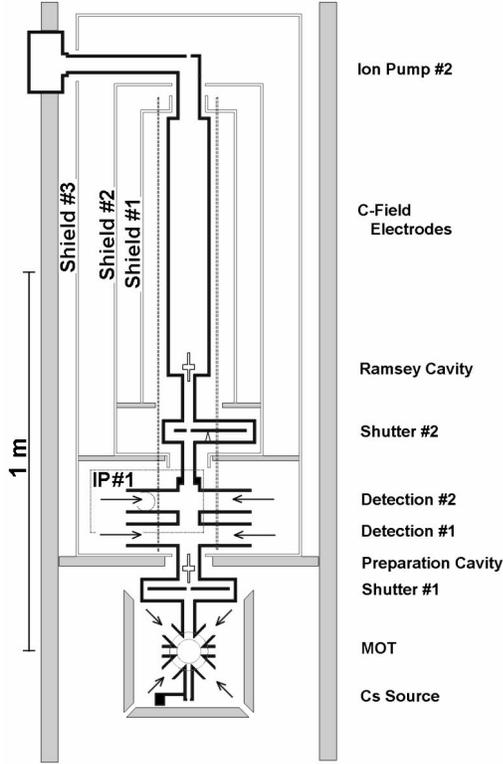
Figure 1. Schematic section of the fountain clock. Dimensions are to scale. IP#1: Ion Pump #1.
