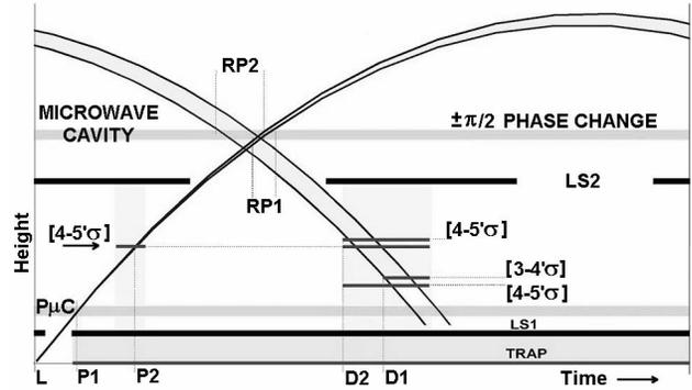
Figure 3. Timing sequence for one launch cycle. LS1 and LS2: light shutters, P $\mu$ C: preparation microwave cavity, RP1 and RP2: Ramsey pulses which may overlap in time, L: launch, P1: microwave preparation, P2: push, D2: detection of  $F = 4$ , D1: detection of remaining atoms.
