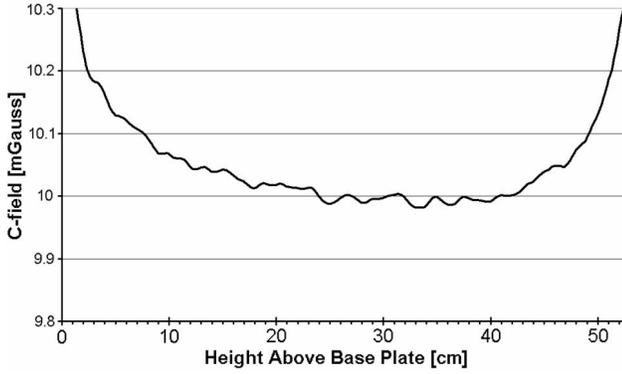
Figure 2. Map of the C-field. The cavity is 2.5 cm above the base plate.
