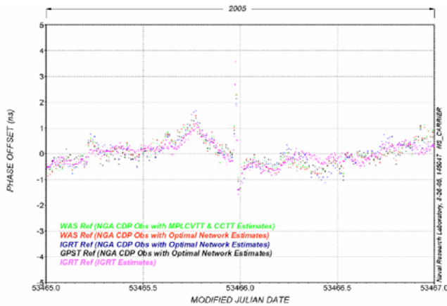
Figure 8. Phase Offset of Navstar 43 tabulated at 15-minute intervals for 4-5 April 2005.
