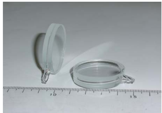
Figure 2. Pyrex glass cells for Cs vapor
