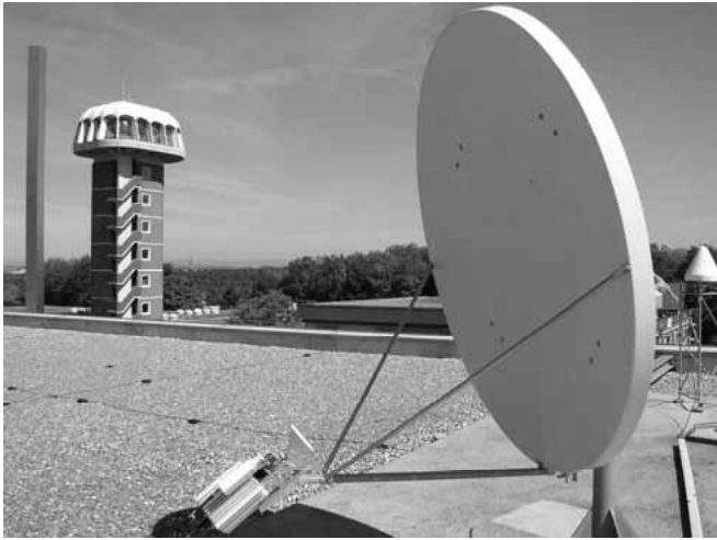
Fig. 6. Photograph of the TWSTFT antenna located on the roof of the new METAS building.
