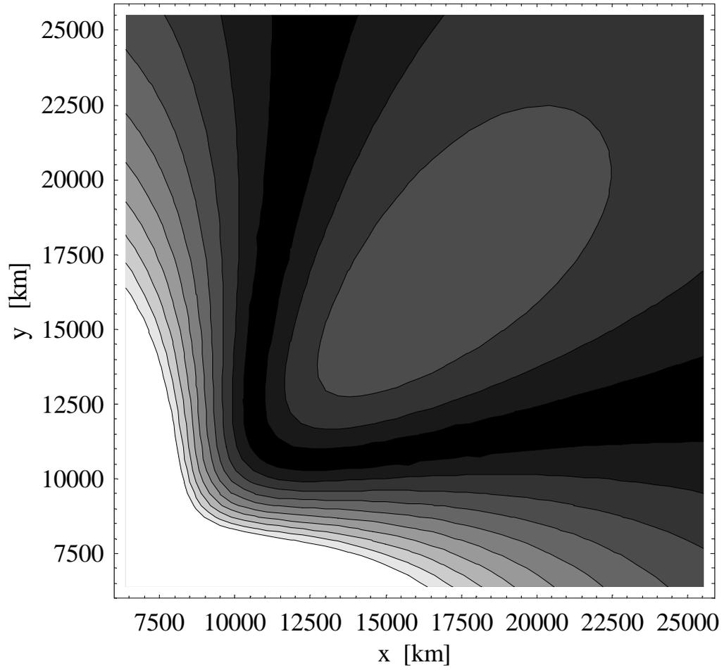
Figure 8: Contours of constant reciprocal position error,  $1/R_{xyz}$ , are shown in the  $x_o - y_o$  plane for  $z_o = R_e/\sqrt{3}$  and  $\sigma_s = 1.0 \mu\text{m}$ . Lighter-shaded areas are smaller values of error  $R_{xyz}$ . The semi-major axis of the LEO satellites is taken to be  $a = 7360$  km and the baselines (satellite pair separation)  $b = 20$  km.
