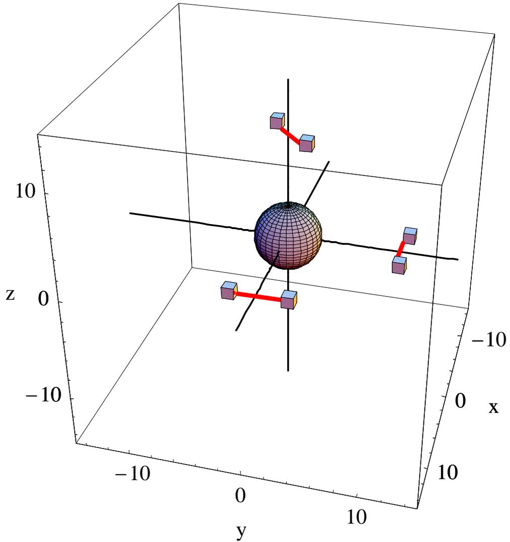
Figure 7: A schematic of the LEO satellite QPS is shown. Pairs of satellites orbiting Earth, shown by connecting lines, form the interferometer baselines of length  $b$ . Example numbers used in this calculation have baseline  $b = 20$  km and LEO satellite semi-major axis  $a = 7360$  km.
