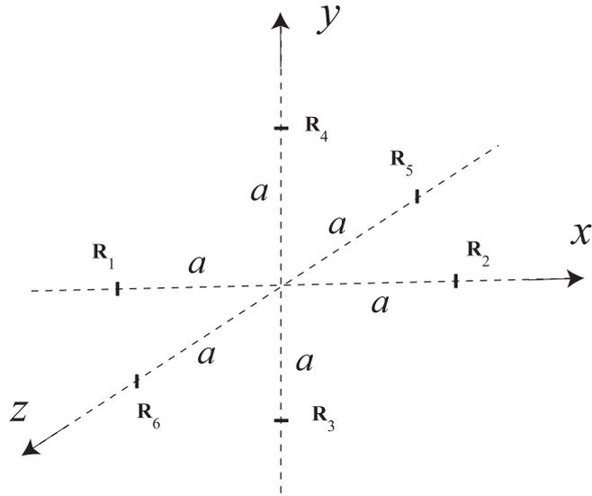
Figure 3: The baselines are shown for a possible terrestrial QPS that might be used on the Earth. The baselines lie along the  $x$ ,  $y$ , and  $z$  axes, are of length  $2a$  and are orthogonal to each other.
