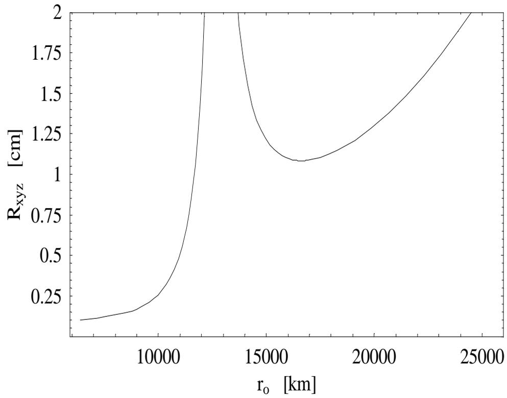
Figure 10: Plot of position error in the radial direction,  $R_{xyz}$  vs.  $r_o$ , where  $r_o = \sqrt{x_o^2 + y_o^2 + z_o^2}$  and  $\sigma_s = 1.0 \mu\text{m}$ . The semi-major axis of the LEO satellites is taken to be  $a = 7360 \text{ km}$  and the baselines (satellite pair separation)  $b = 20 \text{ km}$ .
