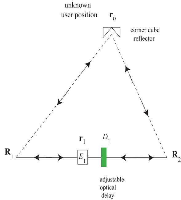
Figure 1: One baseline is shown for the quantum positioning system (QPS). Points  $R_1$  and  $R_2$  on the baseline contribute to the definition of the reference frame for spatial positioning. Box  $E_1$  contains an entangled photon (biphoton) source and 50:50 beam splitter; see Figure 2. The quantity  $D_1$  is a controllable, calibrated optical delay.
