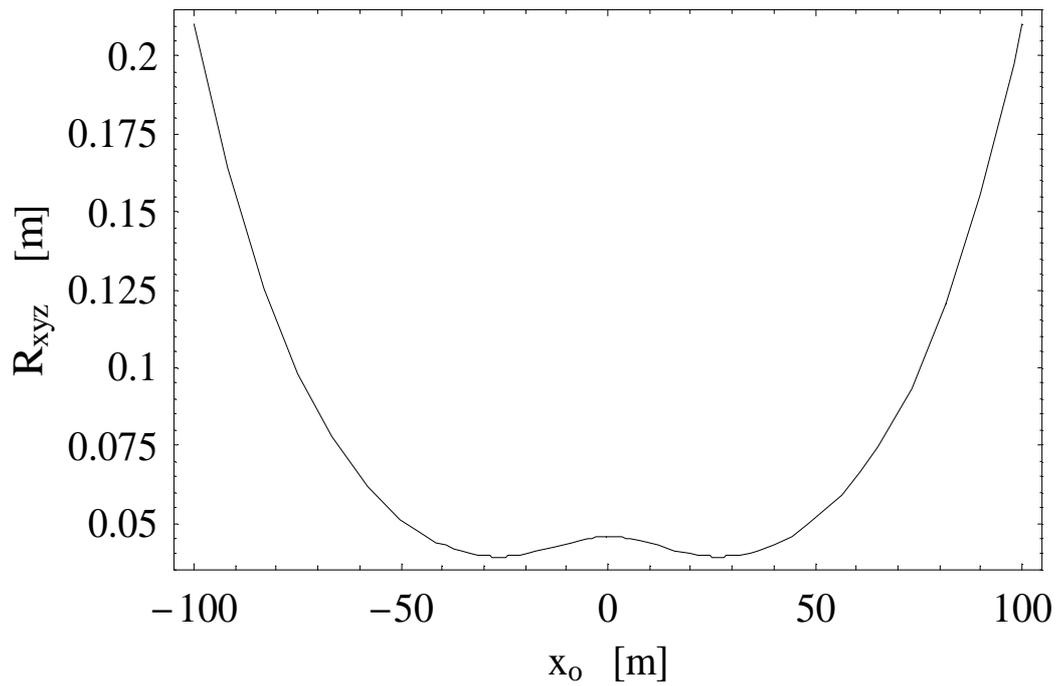
Figure 5: The error  $R_{xyz}$  vs.  $x_o$  is plotted for  $y_o = 30$  m and  $z_o = 100 \text{ m}/\sqrt{3}$ , which corresponds to a line in Figure 4 with relatively small error  $R_{xyz}$ . The same parameters are used in this plot as in Figure 4. Units on both axes are meters.
