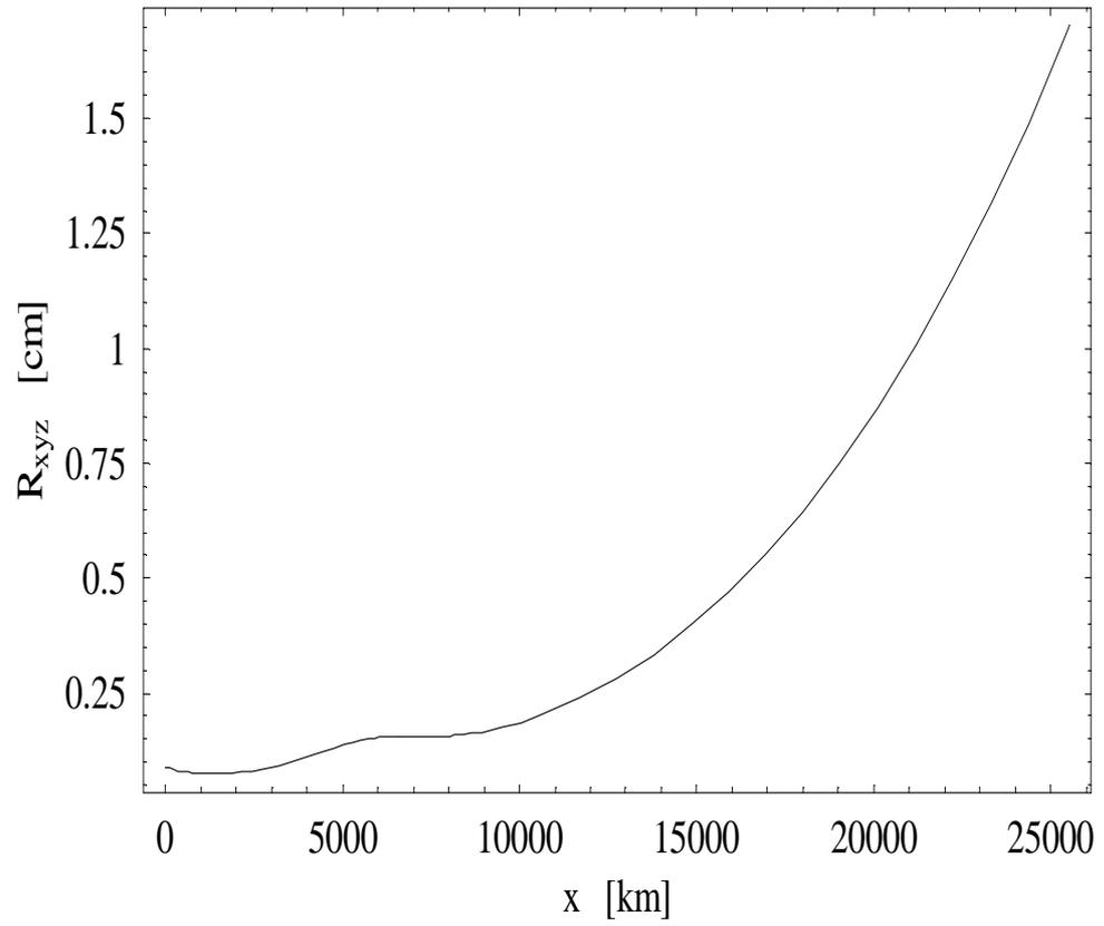
Figure 9: Plot of position error,  $R_{xyz}$  vs.  $x_o$ , shown for  $y_o = z_o = R_e/\sqrt{3}$  with  $\sigma_s = 1.0 \mu\text{m}$ . The semi-major axis of the LEO satellites is taken to be  $a = 7360 \text{ km}$  and the baselines (satellite pair separation)  $b = 20 \text{ km}$ .
