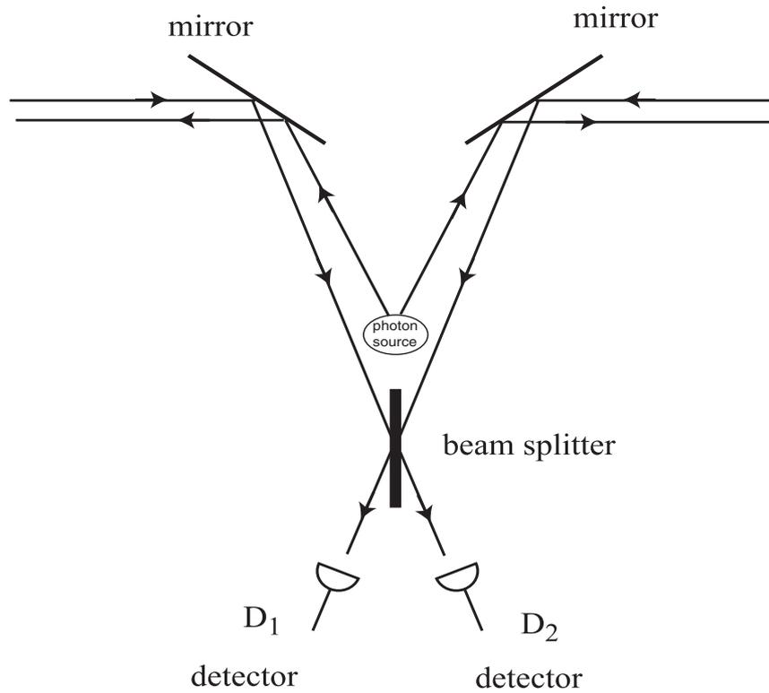
Figure 2: An expanded view of the contents of each of the three boxes  $E_1$ ,  $E_2$ , and  $E_3$ , which are located on the three baselines, one of which is shown in Figure 1. Each box contains an entangled photon (biphoton) source, a 50:50 beam splitter, and two single-photon detectors  $D_1$  and  $D_2$ , to perform photon coincidence counting.
