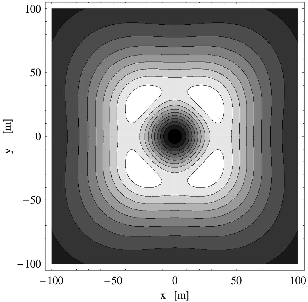
Figure 4: A plot of the contours of constant  $1/R_{xyz}$  is shown in the  $x_o - y_o$  plane at  $z_o = 100/\sqrt{3}$  m. Light-shaded areas are small values of  $R_{xyz}$ . Units on both axes are meters.
