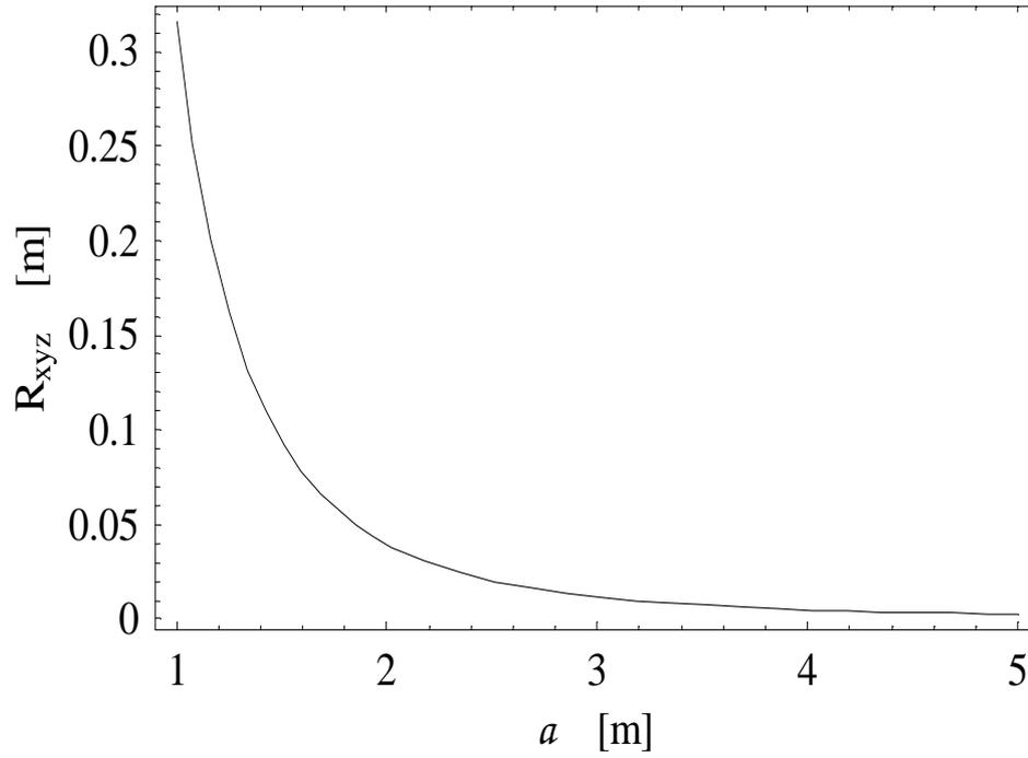
Figure 6: The error  $R_{xyz}$  vs.  $a$  (half the interferometer baseline length) is plotted for  $x_o = y_o = 30$  m, and  $z_o = 100\text{ m}/\sqrt{3}$ , which corresponds to the high-accuracy light-shaded region in upper right of Figure 4. Units on both axes are meters.
