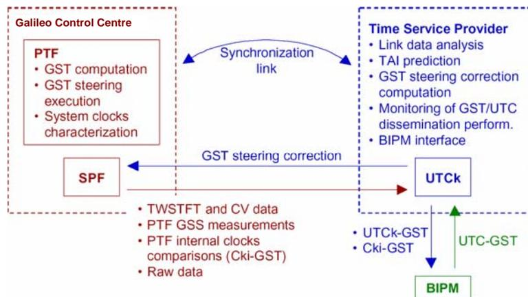
Figure 2. Task allocations and links between PTF (left) and GTSP (right) after [1]. SPF = “Service Products Facility”. I/F to GPS (USNO) not shown here.
