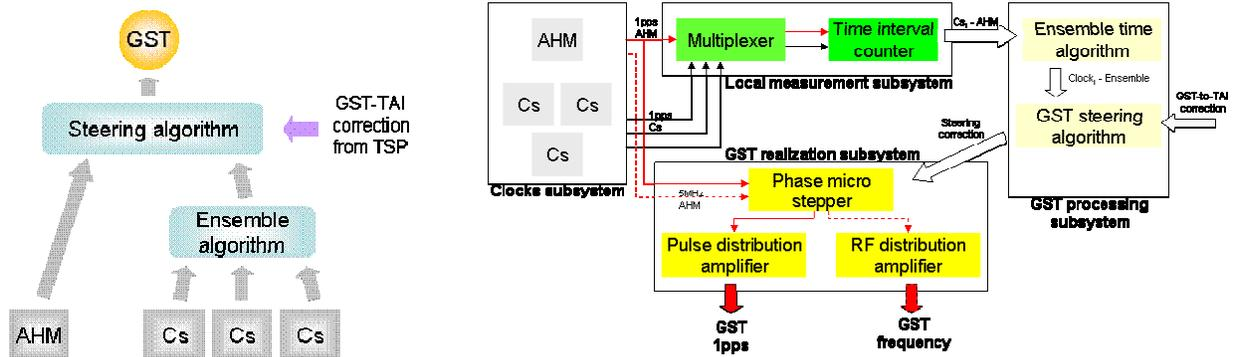
Figure 4. GST generation/steering chain: conceptual level (left), physical level (right).
