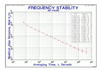
The following plot of two active hydrogen masers (Sigma Tau vs. KVARZ) shows stability below 2×10<sup>-15</sup>
