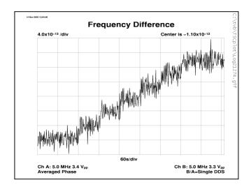
It can be seem from the plot that a total of six steps increase the frequency by about  $2x10^{-12}$ . Since each step is 1000 octal (512 decimal), the resolution of the DAC is  $6.6 \times 10^{-16}$  per bit. The 3-month trend was
