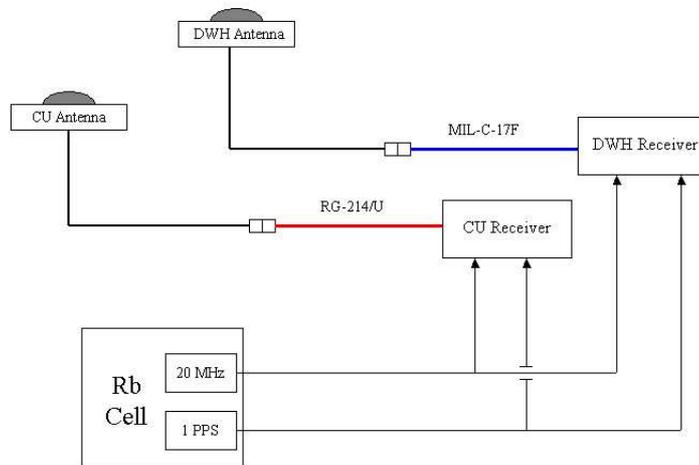
Figure 4: Short-baseline experimental setup.
