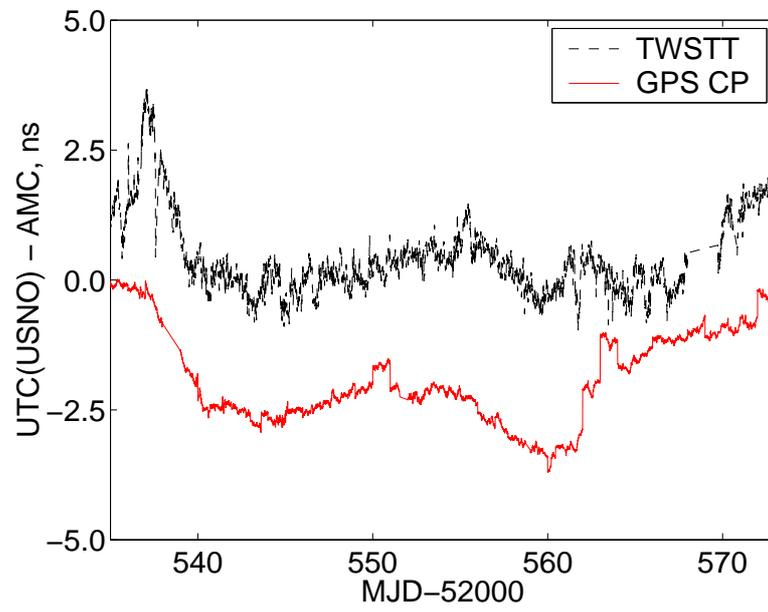
Figure 7: Comparison of TWSTFT and GPS CP estimates of UTC(USNO)-AMC.
