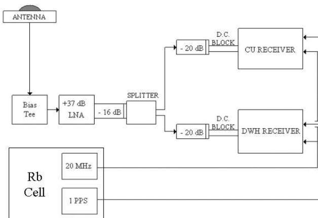
Figure 2: Zero-baseline experimental setup.
