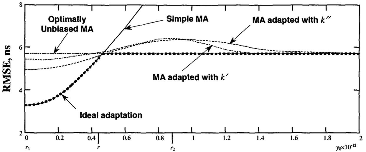
Figure 3. RMSE of the simple MA, optimally unbiased MA, and adapted MA filter for the discrete time error linear process (1) with  $x_0 = 0$ ,  $y_0 = \text{var}$ ,  $D = 0$ ,  $\Delta = 100$  sec,  $\sigma_n = 40$  ns, and  $\theta = 6$  hours ( $N = 216$ ).
