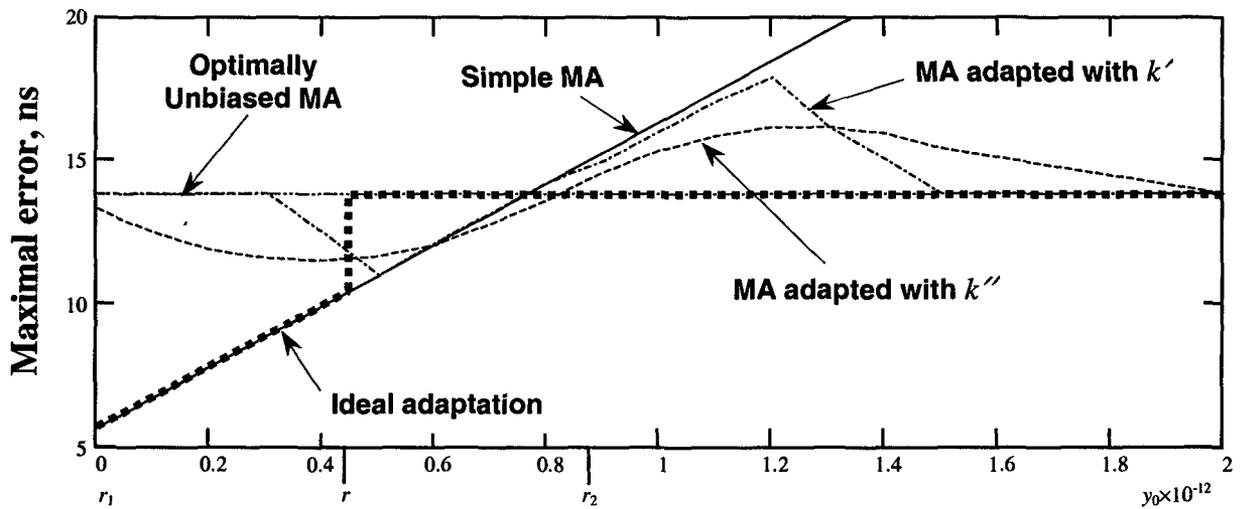
Figure 4. Maximal error of the simple MA, optimally unbiased MA, and adapted MA filter for the discrete time error linear process (1) with  $x_0 = 0$ ,  $y_0 = \text{var}$ ,  $D = 0$ ,  $\Delta = 100$  sec,  $\sigma_n = 40$  ns, and  $\theta = 6$  hours ( $N = 216$ ).
