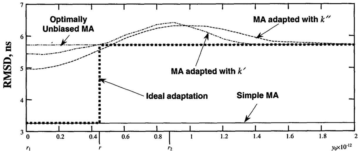
Figure 2. RMSD of the simple MA, optimally unbiased MA, and adapted MA filter for the discrete time error linear process (1) with  $x_0 = 0$ ,  $y_0 = \text{var}$ ,  $D = 0$ ,  $\Delta = 100$  sec,  $\sigma_n = 40$  ns, and  $\theta = 6$  hours ( $N = 216$ ).
