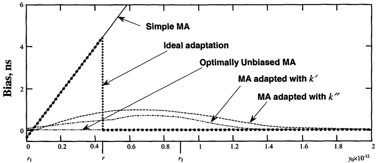
Figure 1. Bias produced by the simple MA, optimally unbiased MA, and adapted MA filter for the discrete time error linear process (1) with  $x_0 = 0$ ,  $y_0 = \text{var}$ ,  $D = 0$ ,  $\Delta = 100$  sec,  $\sigma_n = 40$  ns, and  $\theta = 6$  hours ( $N = 216$ ).
