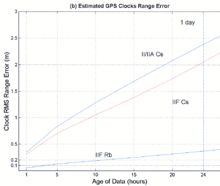
Figure 2. (a) Allan variances of GPS Block IIF, and (b) estimated IIF clocks Range Error.
