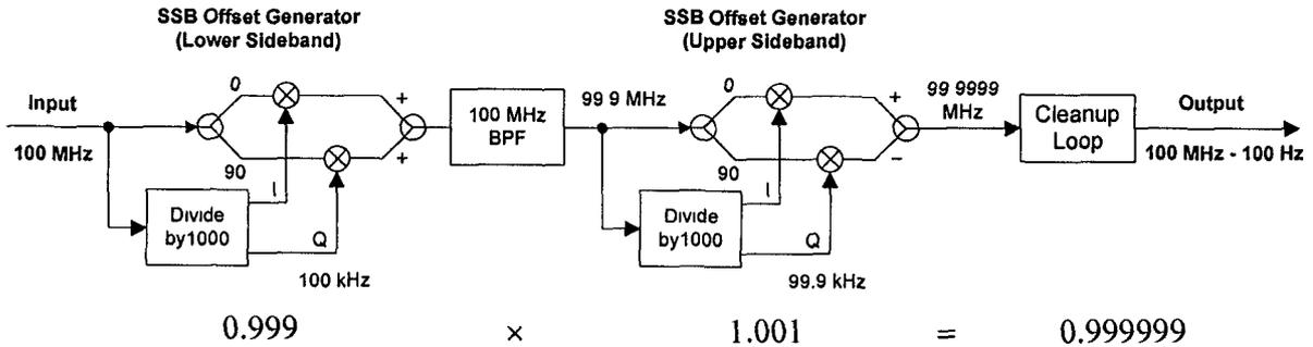
Fig. 2. Offset generator for lowering a 100-MHz source by 100 Hz. Two cascaded single-sideband mixers are followed by a phase-locked cleanup loop with a low-noise VCXO.
