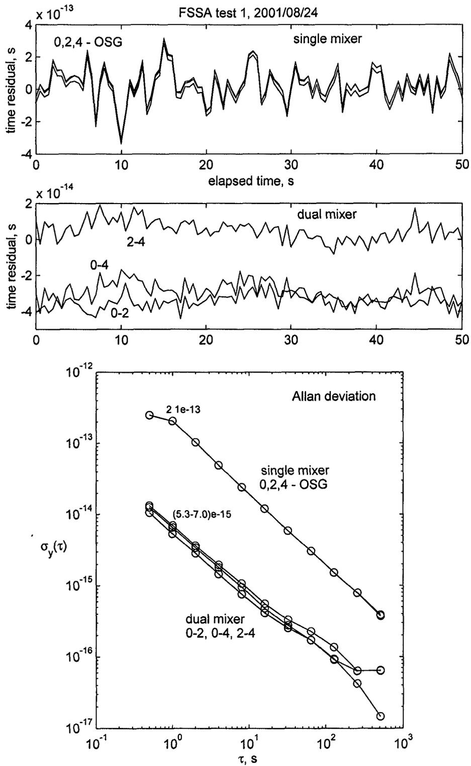
Fig. 4. Results of the first noise floor test
