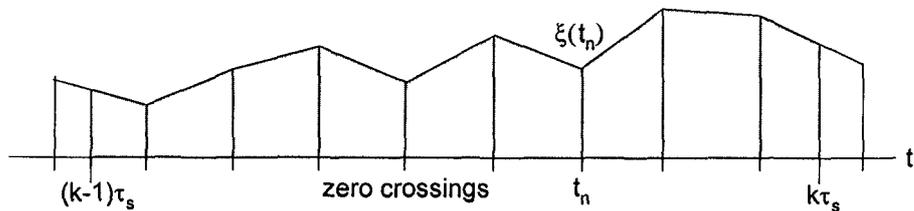
Fig. 3. A beat-note zero crossing at  $t_n$  gives rise to a phase residual  $\xi(t_n)$ . Between the zero crossings, the phase is interpolated linearly. The average phase for the interval  $[(k-1)\tau_s, k\tau_s]$  is the shaded area divided by  $\tau_s$ .
