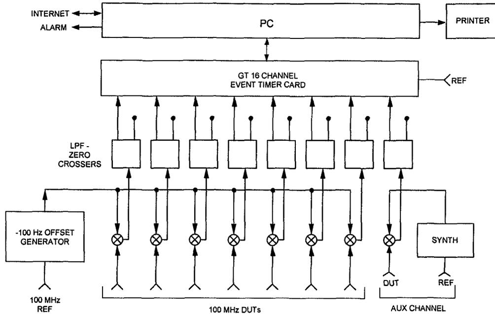
Fig. 1. Stability analyzer architecture
