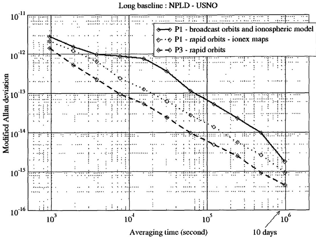
Figure 4. Frequency stability corresponding to Figure 3.
