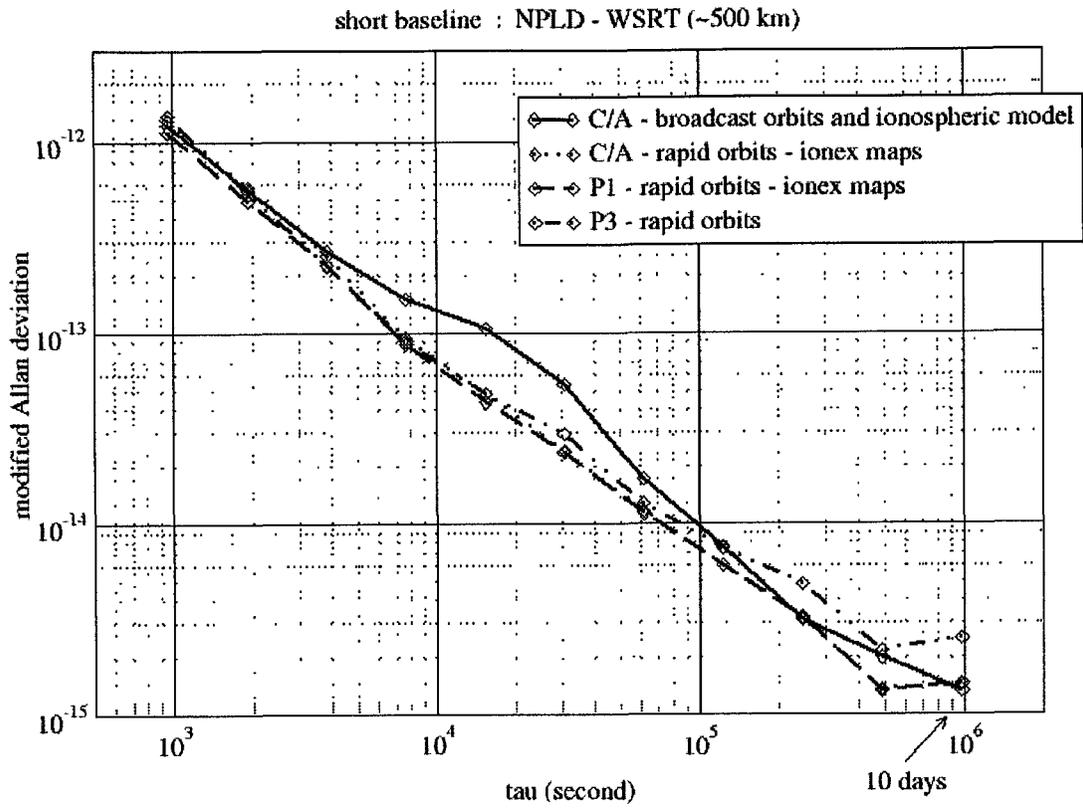
Figure 2. Frequency stability corresponding to Figure 1.
