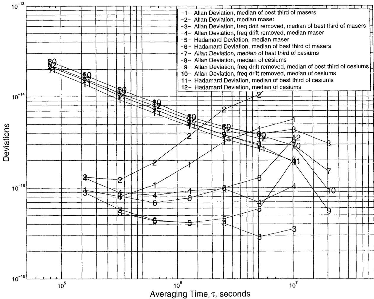
Figure 5. Postprocessed timescale frequency stabilities from N-cornered-hat analyses using editing criteria Set #3. The high values for curves "1" and "2" are due to the analyses systematically overstating the uncertainties of the lower-sigma clocks.
