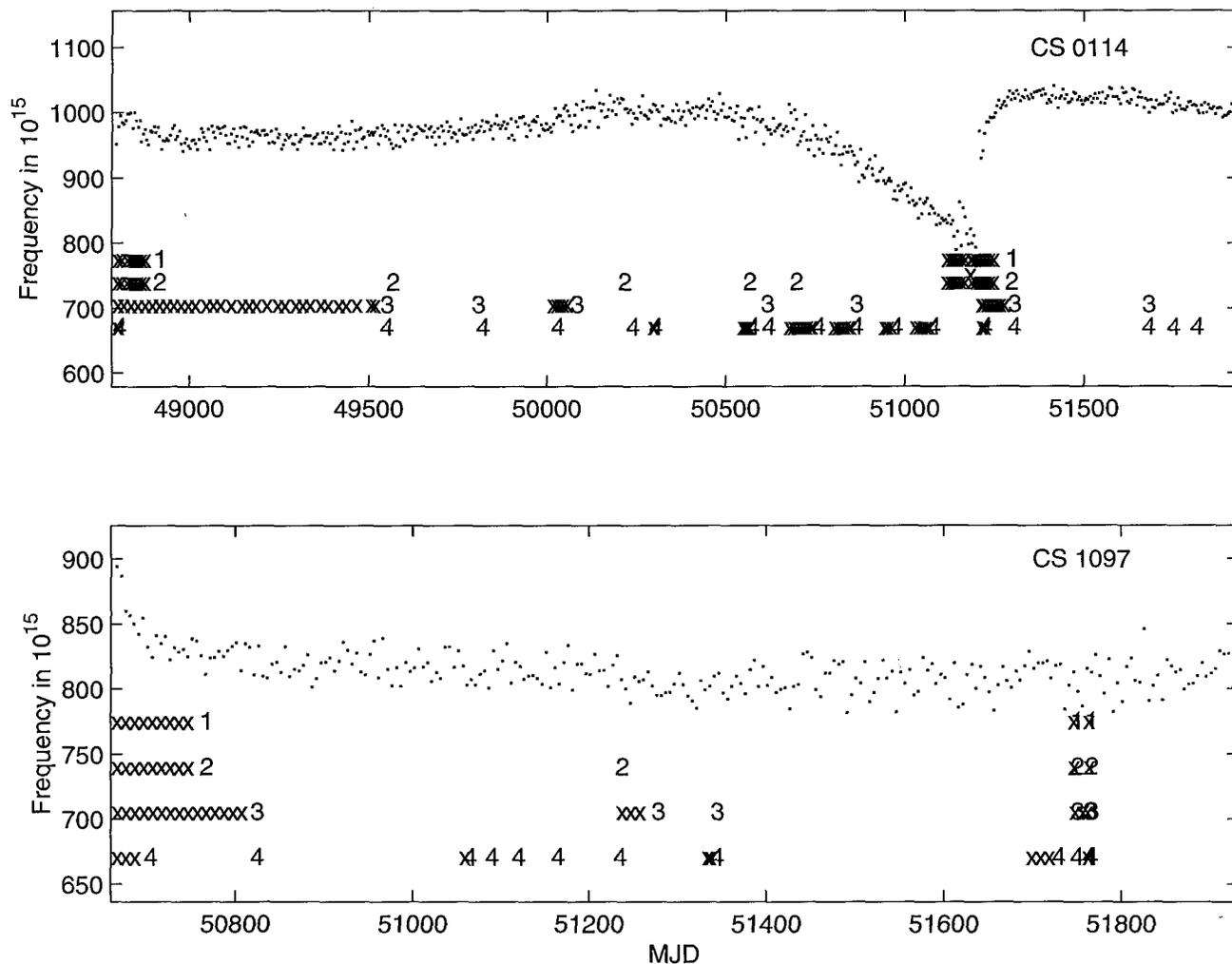
Figure 1. The frequencies of two cesium standards referenced to the cesium mean timescale, with the times of clock breaks determined by the four different sets of criteria indicated by "1," "2," "3," or "4." "x"'s in the row dedicated to a particular criteria set indicates that data were deweighted from that point on until the next clock break.
