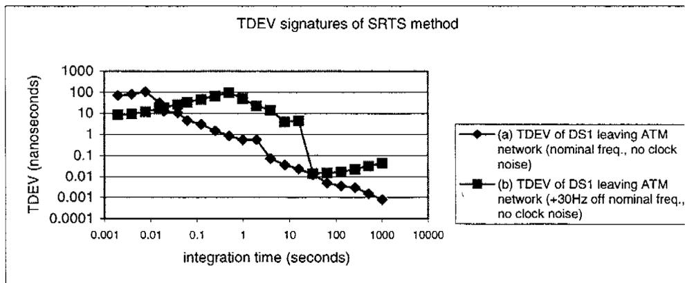
Figure 4. TDEV of DS1 leaving ATM network when there is no noise in any clock:
