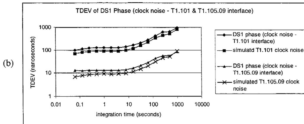
Figure 8. TDEV of simulated DS1 resulting from clock noise
