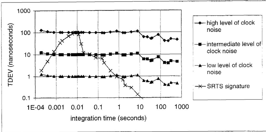
Figure 9. TDEV of various levels of source noise.
