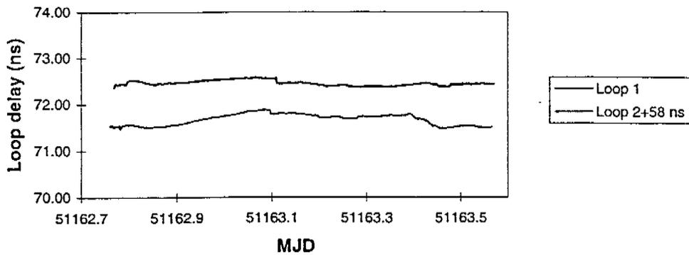
Figure 13. Measurements for two downlink characterization loops taken using the Satre modem.
