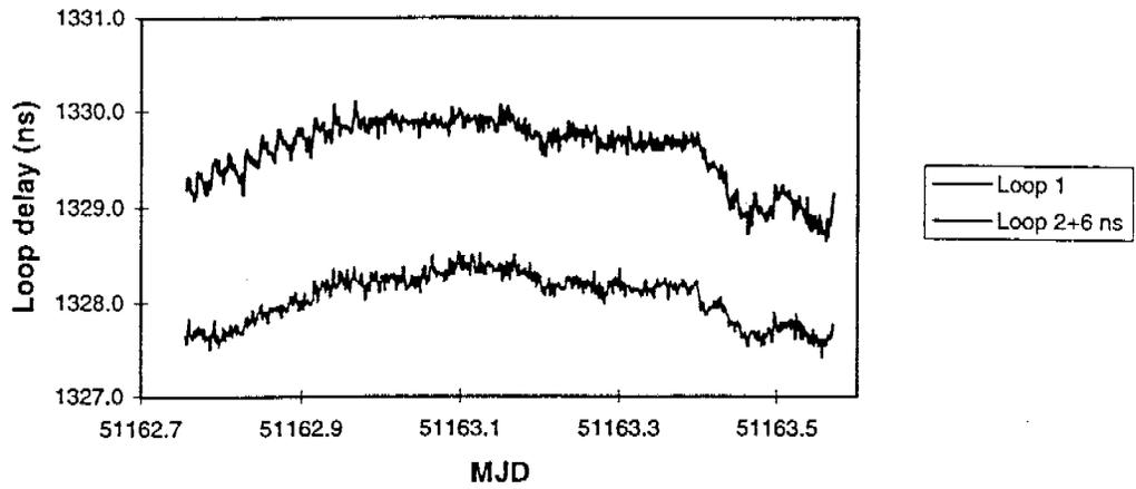
Figure 12. Measurements for two downlink characterization loops taken using the Mitrex modem.
