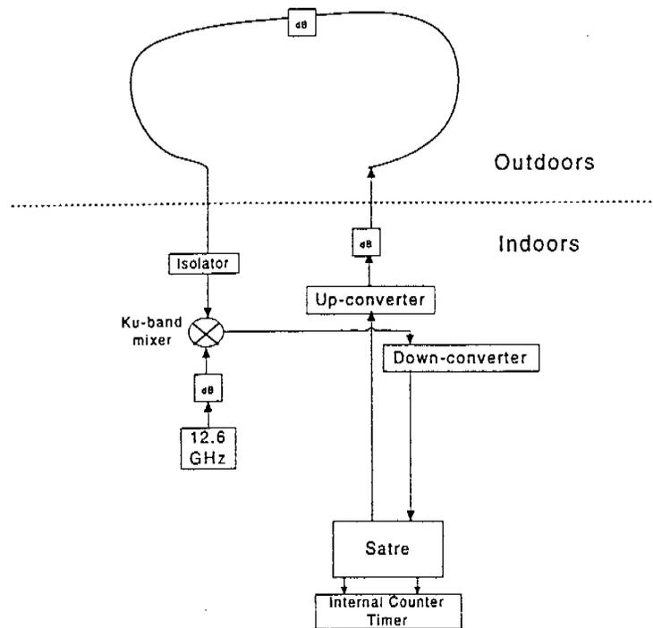
Figure 8. Configuration used to investigate Ku-band signal delay variations in PTFE cables.
