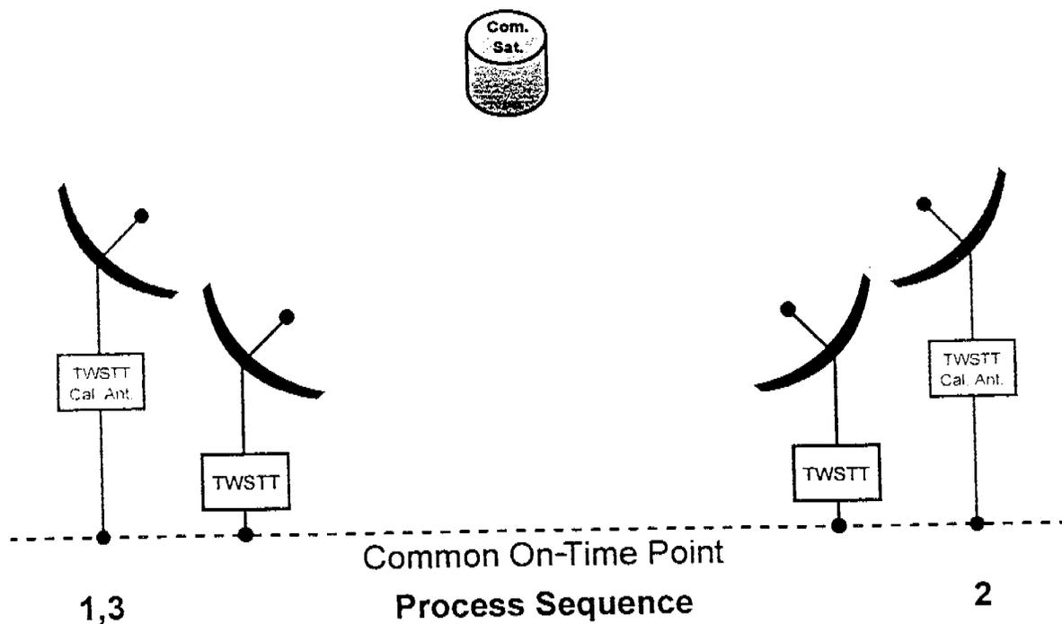
**Fig. 9 GPS Receiver Link Calibrated by Co-Located TWSTT Method**
