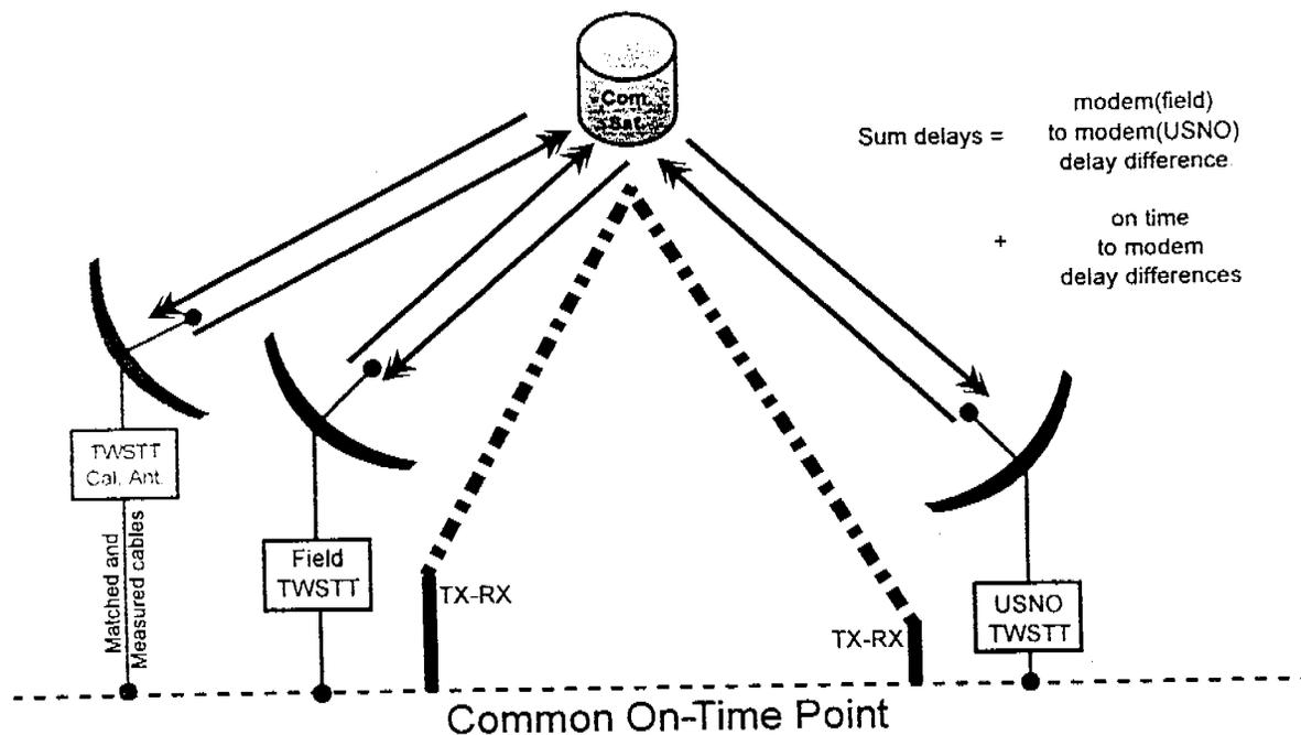
**Fig. 8** TWSTT Link Calibrated by Co-Located TWSTT Method
