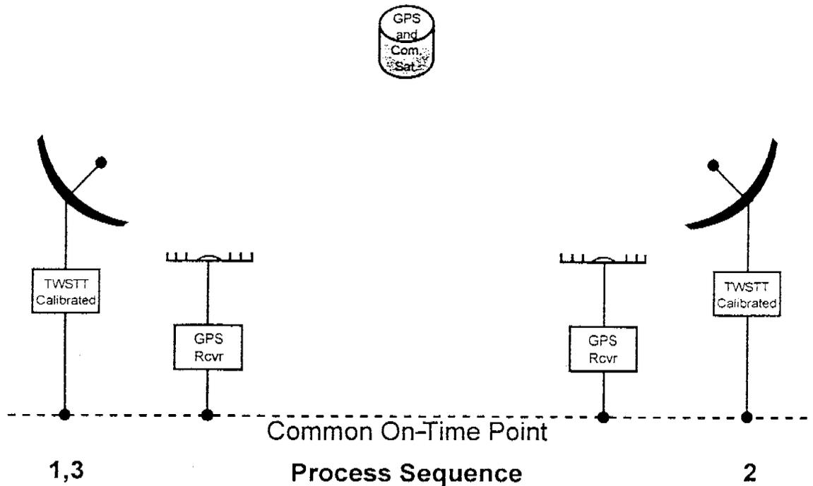
**Fig. 10 USNO - NRaD Syntonization and Single-Shot Synchronization**
