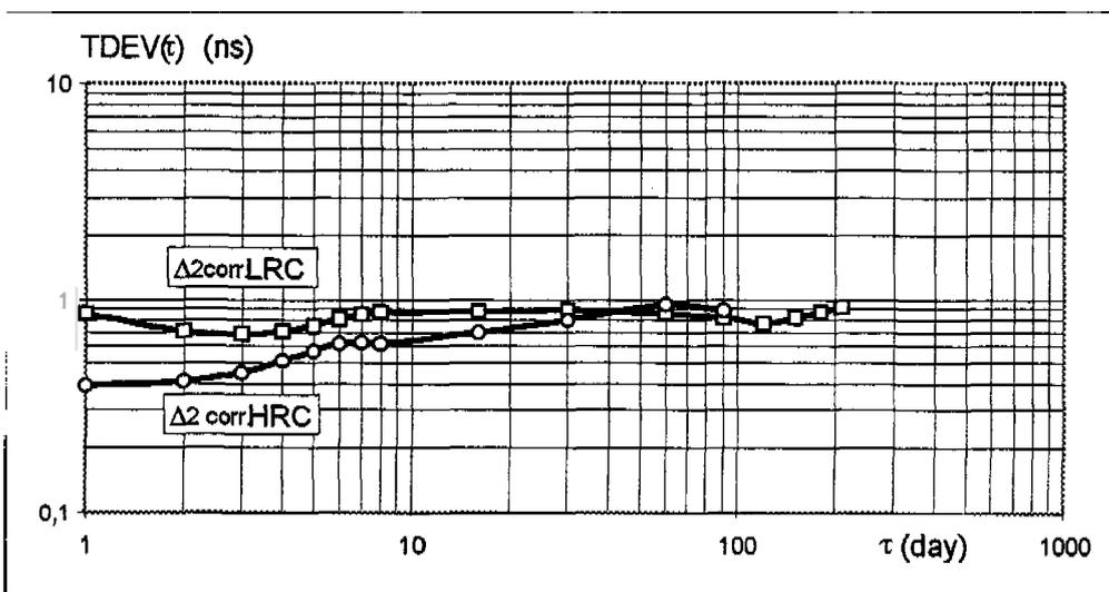
Fig. 6 displays the plots of  $TDEV(\tau)$  of corrected propagation delay of the loop 2 calculated from the data measured by low resolution counters ( $\Delta_{2 \text{ corr}}$  LRC) and by high resolution counters ( $\Delta_{2 \text{ corr}}$  HRC).
