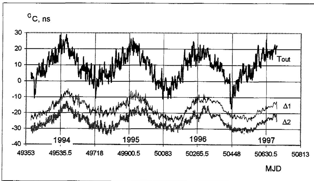
Fig.2 This figure shows the plots of relative summary propagation delay  $\Delta_1$  of the loop 1 created by links 0 and 1, and  $\Delta_2$  of the loop 2 created by links 0 and 2. The third plot displays the mean daily outdoor temperature  $T_{out}$  in Prague.
