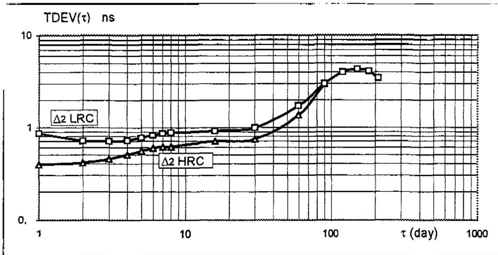
displays the plots  $TDEV(\tau)$  of uncorrected propagation delay of the loop 2 calculated from the data measured by low resolution counters ( $\Delta_2$  LRC) and by high resolution counters ( $\Delta_2$  HRC).
