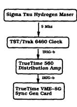
BCD timecode can be read with essentially zero latency. Two sync-gen cards are installed in the NTP server. Each card is synchronized to one of USNO Master Clocks #1 or #2. Each Master Clock is a Sigma Tau Hydrogen Maser providing 5Mhz to TST/Trak 6460 Clocks, which generate IRIG-B timecode that is distributed by TrueTime 560 distribution amps with parallel output to multiple NTP server inputs.
