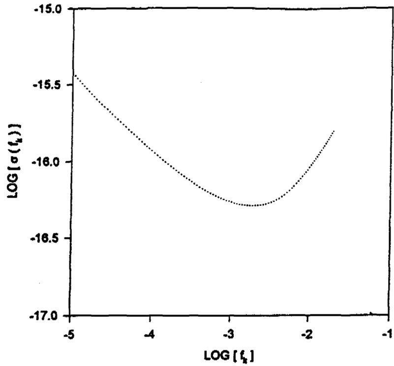
Figure 3: The sensitivity curve achievable with the Cassini Doppler data during the first solar opposition. The distance to the spacecraft is about  $L = 5.5$  AU, and the corresponding fundamental frequency  $f_0$  is equal to  $4.5 \times 10^{-5}$  Hz.
