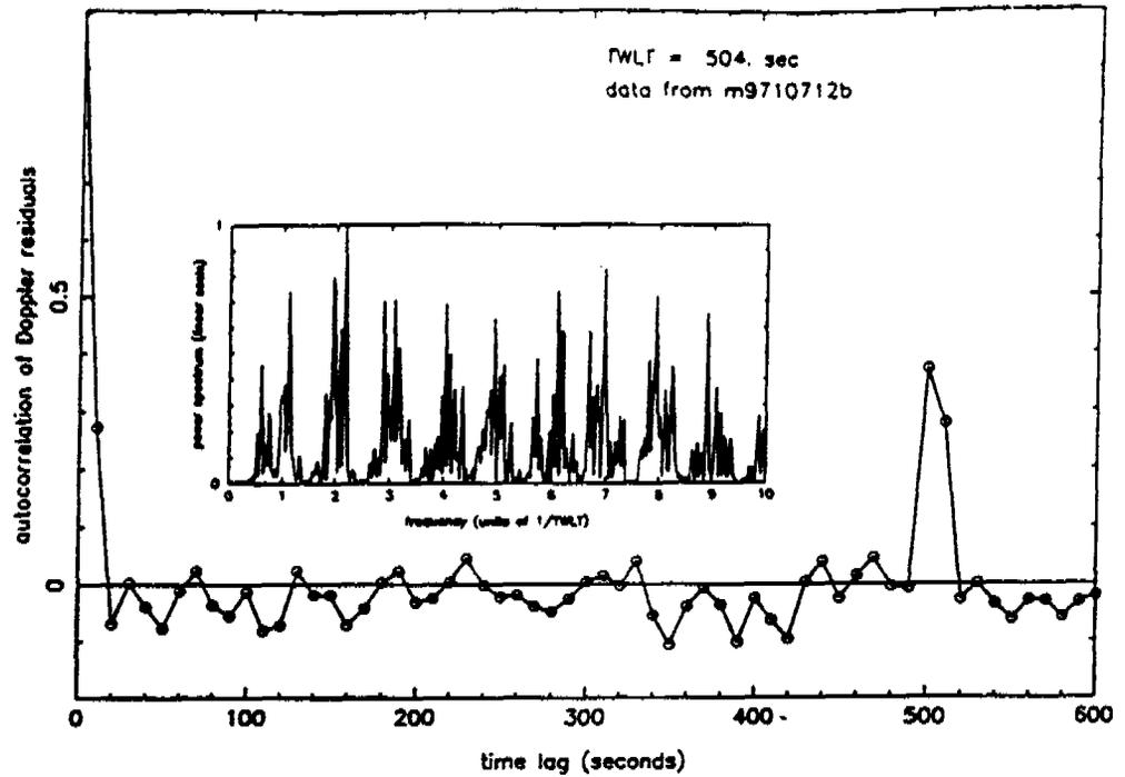
Figure 1: The temporal autocorrelation function of 10-second time resolution Mars Global Surveyor (MGS) data taken on April 17, 1997, when the two-way light time  $2L/c$  was equal to 504 seconds. The inset plot shows the power spectrum, with frequency scale marked in units of  $1/2L$ .
