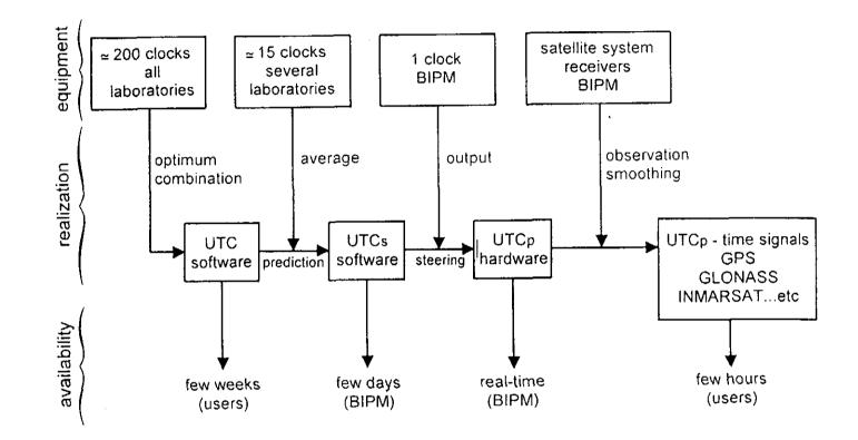
Figure 1. Block diagram of the realization of the real-time prediction of UTC, UTCp
