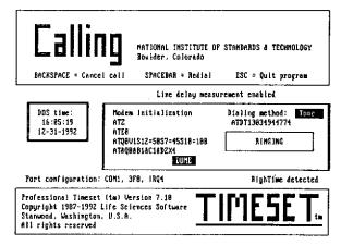
Figure 4. Modem initialization and dialing the NIST with line delay request.
