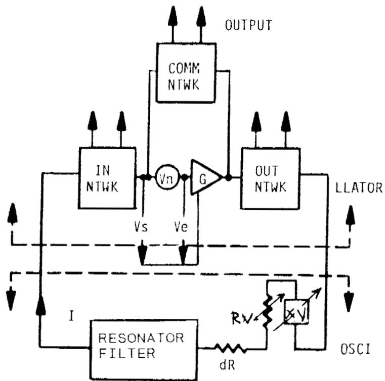
Figure 2: Real Oscillator, Special Case, N Configuration
