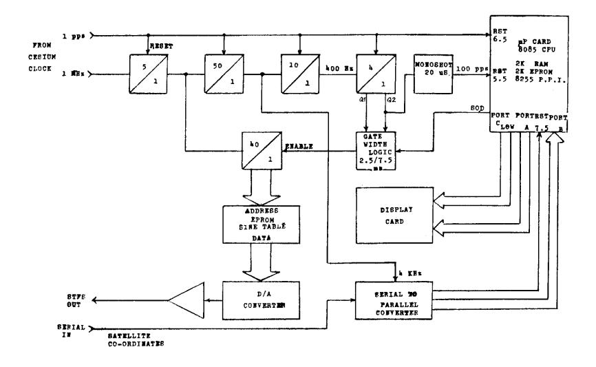
Figure 4. Block Diagram of the STFS Format Generator
