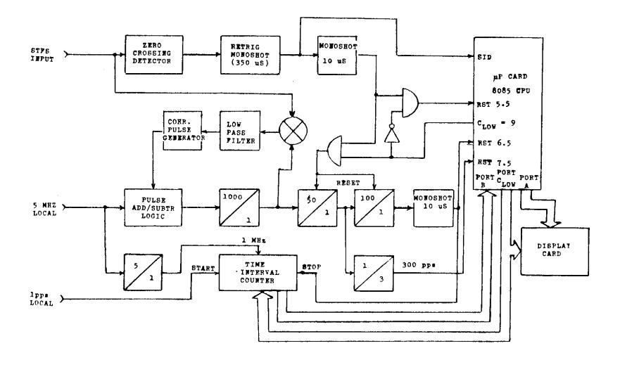
Figure 6. Block Diagram of the STFS Decoder
