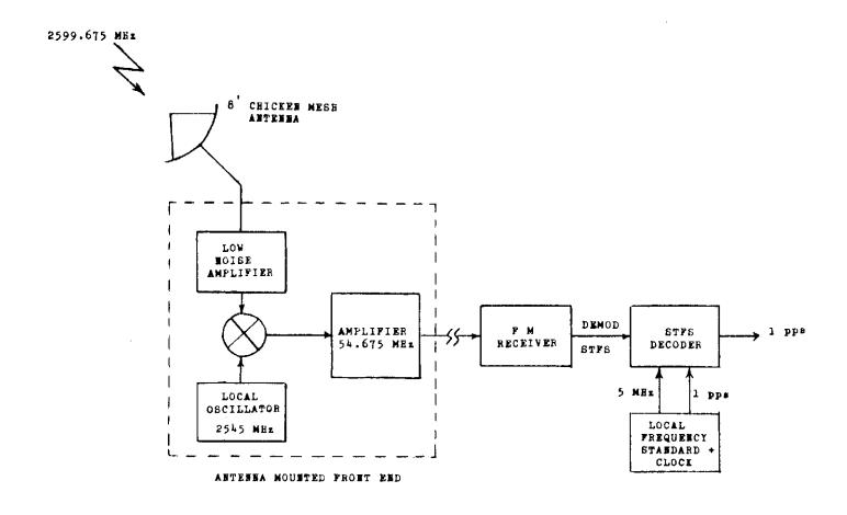
Figure 5. Block Diagram of the Receiving Setup
